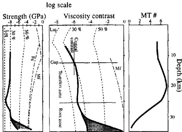
**Fig. 3.** Evolution of physical parameters in and around the Closepet granite, at the time of its arrival at a given depth. Left: Strength under strike-slip deformation; Middle: viscosity contrast between granitic magmas and gneissic basement; Right: MT# (Olsen and Baumgartner, 2000), which is an estimation of the relative importance of mass transfer vs. liquid percolation in a magmatic suspension.
