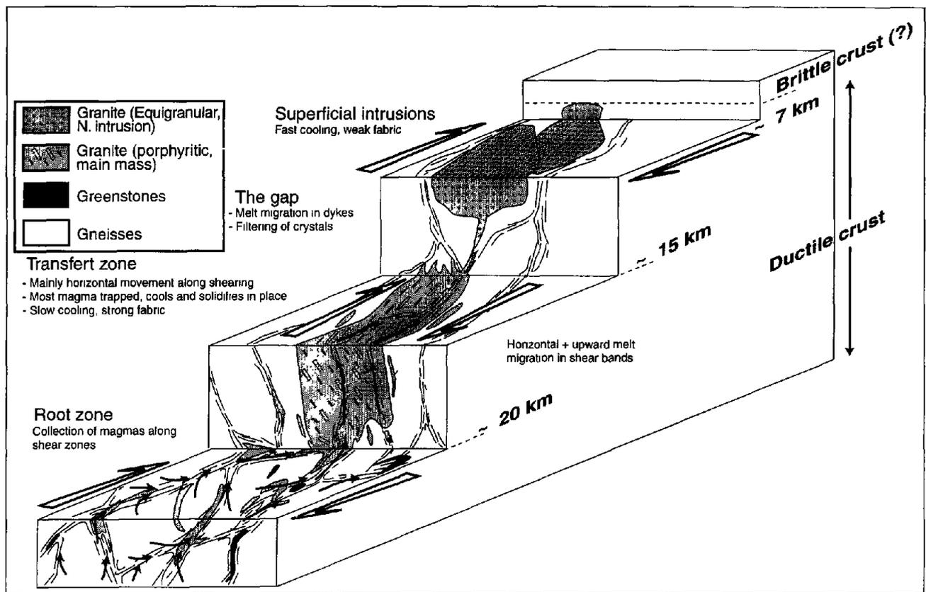
Fig. 2. Sketch drawing of the emplacement mode and strain partitioning in the Closepet granite at contrasted structural levels (Moyen, 2000). Comments in the text and on the figure. Black, thin arrows: melt movement; white, large arrows: kinematics of deformation.
